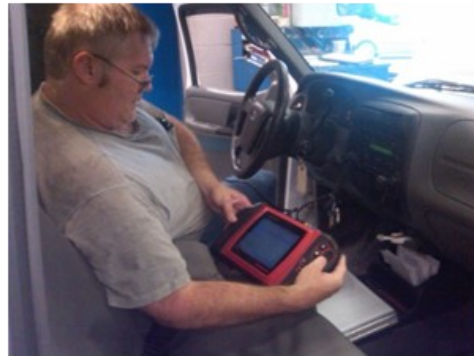
Billy Freeman, a fourth semester Automotive Service Technology student analyzes engine performance data using a handheld computerized diagnostic instrument connected to the vehicles on-board electronic system.
